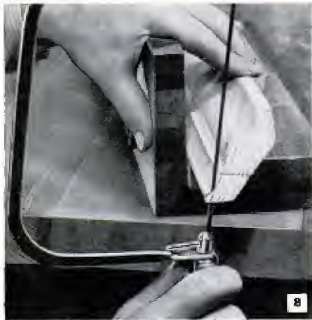
Above, making the cope cut after mitering the end of the molding. Miter cut is guide for the cope cut. Below, checking the accuracy of the joint after coping. When coping the stock is slightly undercut
